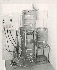
Zymurgy reader Dion Hollenbeck's RIMS system. The temperature controller cabinet is homebuilt with parts mostly from Omega (PID controller and SSRs). The pump is from March, the stand is completely homebuilt. The two 6,500 watt heater elements are from Grainger. All parts of the system are connected with Hansen.
